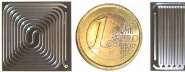
MEMS for pre concentration and gas chromatographic separation
