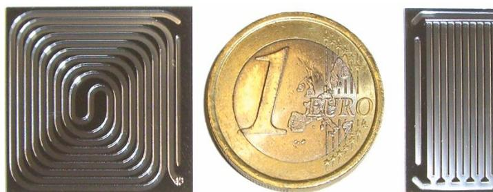
Figure 1 - Pre-concentrator and MEMS chromatographic gas column
