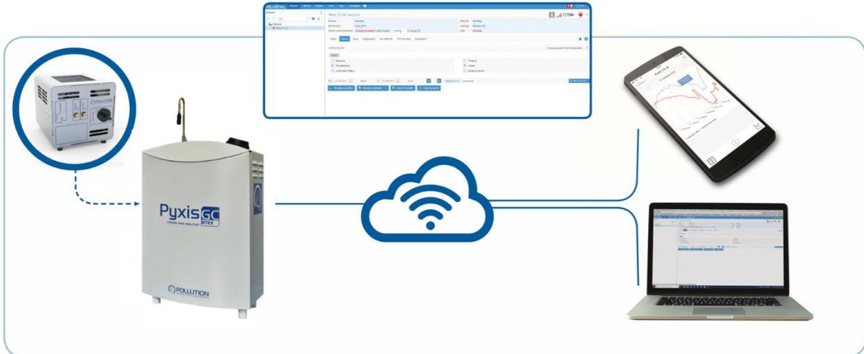
Figure 6 - Cloud System for PyxisGC BTEX
