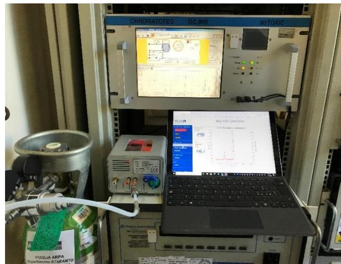
Figure 2 - Installation of the PyxisGC BTEX in the cabin
